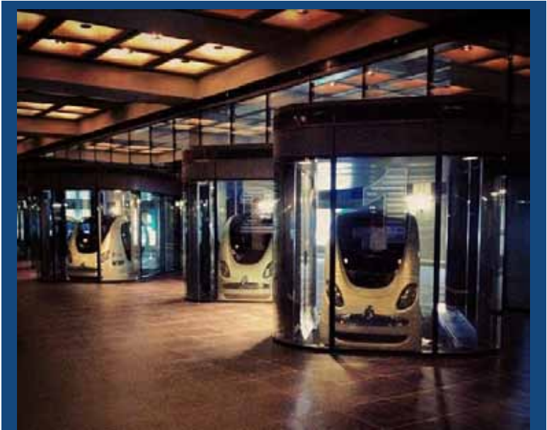
Figure 3-2. 2getthere PRT Vehicles in Station
