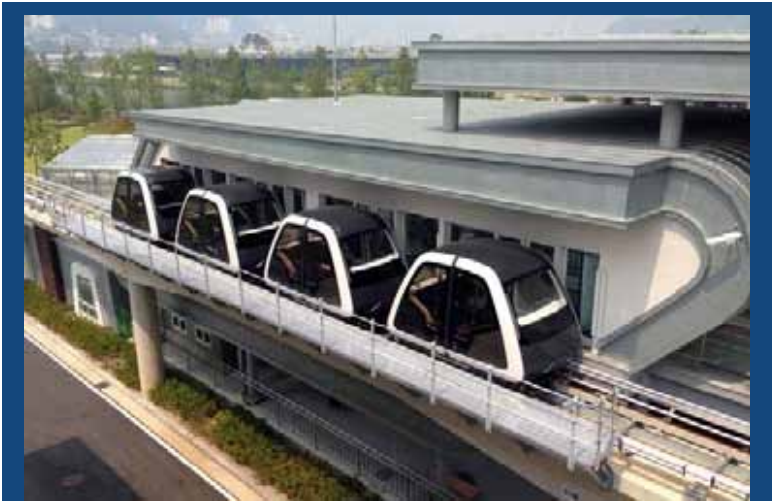
Figure 3-3. Vectus PRT Vehicles in Station
